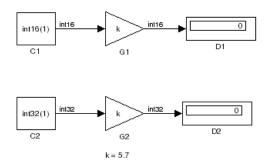
The two Gain blocks in this model both use k, a tunable parameter of unspecified type, as their gain parameter. Computing the outputs of the blocks requires that the gain parameter be of types int16 and int32, respectively. In Release 13, Simulink regards the data type of k to be double and the Gain
