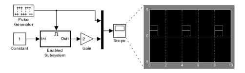
Simulink computes the outputs of the Constant block and Gain Block only when the Enabled Subsystem executes (i.e., at time steps 0, 4, 8, and so on). This is because the output of the Constant block is required and the input of the Gain block changes only when the Enabled Subsystem executes. When CE behavior is off, Simulink computes the outputs of the Constant and Gain blocks at every time step, regardless of whether the outputs are needed or change.
