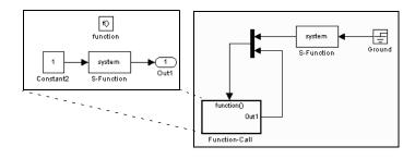
Such models cannot be correctly simulated. Accordingly, Simulink now displays an error message when you attempt to run or update a diagram containing function-call cycles.
