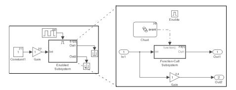
In this example, the previous release of Simulink executed the Stateflow chart that calls the function-call subsystem before it executes the blocks that compute the function-call subsystem's input. In other words, the function-call subsystem runs before its input is ready, which is an error. This release fixes this problem.
